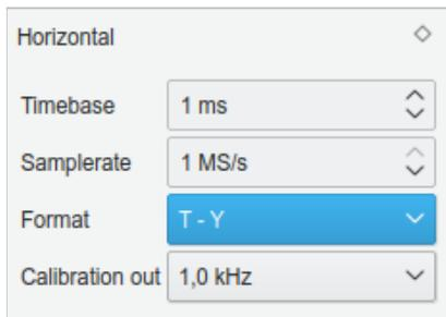
The displayed time range of the trace can be selected by **Timebase** between 10 ns/div and 100 ms/div in 1/2/5 steps.
