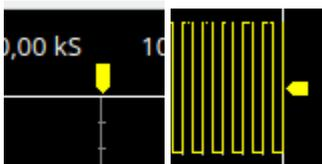
The trigger level (voltage) can be selected by dragging the small colored (e.g. yellow) arrow to the right of the recording window. The trigger position on the screen can be selected by dragging the colored (e.g. yellow) arrow at the top of the window.
