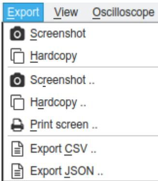
The Export CSV function allows to store the measured samples and the resulting spectral values as a \*.csv file (comma separated values). All 20000 voltage samples as well as all 10001 calculated spectral components of all active channels are stored.
