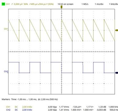
A zoomed screen with 1:1 ratio of Zoom:main can be scaled to double height, configuration: Oscilloscope/Settings/Scope
