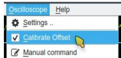
For safety reasons, calibration will not be carried out if the input signals are too noisy or have a too big offset. If successful, the calibration values are stored in the EEPROM when the oscilloscope is switched off. The next time the oscilloscope is started, the calibration is read and used until the next change.
